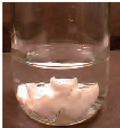
Krytox® grease in hydrocarbon solvent is not dissolved.
