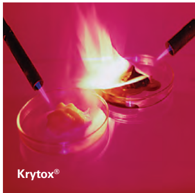
Hydrocarbon-based lubricants burn; Krytox® does not.
