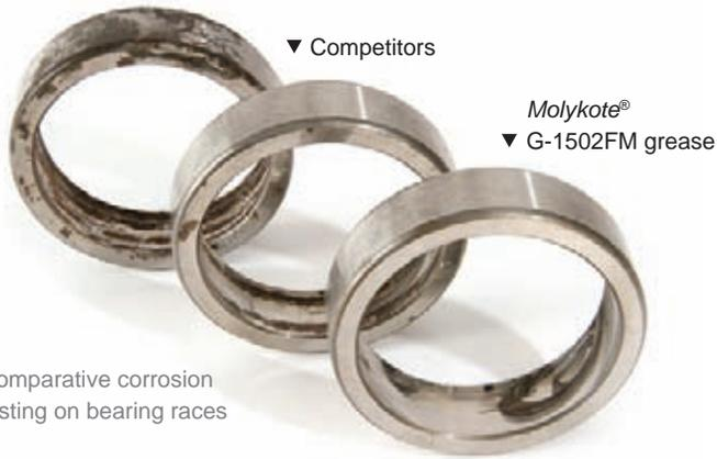
Comparative corrosion testing on bearing races
