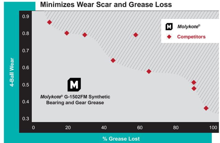
NOTE: All four-ball wear scar results are recorded as average results of vertical and horizontal scars from three different balls.
